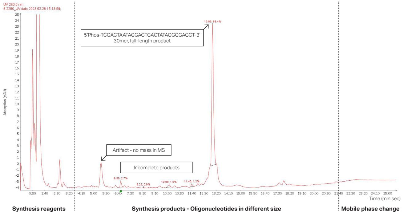
Figure 5: Chromatogram of reverse HPLC collecting absorption at 260 nm overtime
